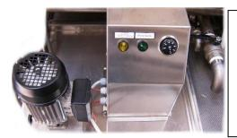
Loading of the oil into the fryer automatically (controlled by MAX and MIN levels) or manual. If the oil level exceeds the set one, the overfull drains the excess oil into the recovery tank. Maintaining a certain temperature through one resistance in the oil recovery tank so that the oil doesn't solidify.
